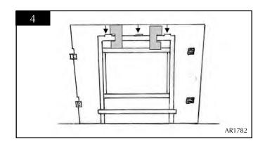
2.5 Remove the back panel and drill the seven fixing holes, push the rawlplugs into the holes and secure the back panel to the wall with the screws supplied.
